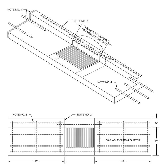
NOTE NO. 1 DRILLED IN DOWELS & NO. 4 REBAR OR 3/4" EXPANSION WITH 3/4"x24" SMOOTH DOWELS & 16" PAPER TUBES, OR 1/2" REBAR DRILLED WITH 5/8" BIT. DOWELS SHALL BE GREASED THE FULL LENGTH. ALL PAPER TUBES SHALL BE PLUGGED OR CRIMPED ON OPEN END AS DETERMINED BY THE ENGINEER. ALL JOINTS SHALL BE SEALED.
